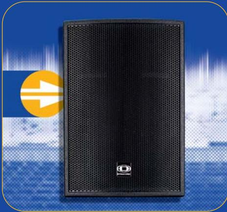
The **MADRAS M 15** is equipped with an Electro-Voice ND-6 neodymium driver with a 3-inch voice coil for the HF range and a 15" Electro-Voice EVX 155 for the LF range. These are driven by the integrated crossover (124 Hz, Linkwitz-Riley 24 dB/Octave) with signal processing and a two-way power stage with separate LF- and HF-channels. A slide switch allows you to select between "Full-range" and "Mid-High" operation modes.
